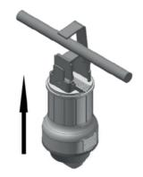
Push indicator upward to the (live) line to clamp it
